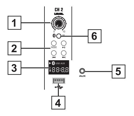
**B1** - Volume control knob **B2** - Command panel of the reader: MODE:
