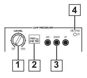
**A1** - Volume control knob for the HF module. From OFF to full power (clockwise).
